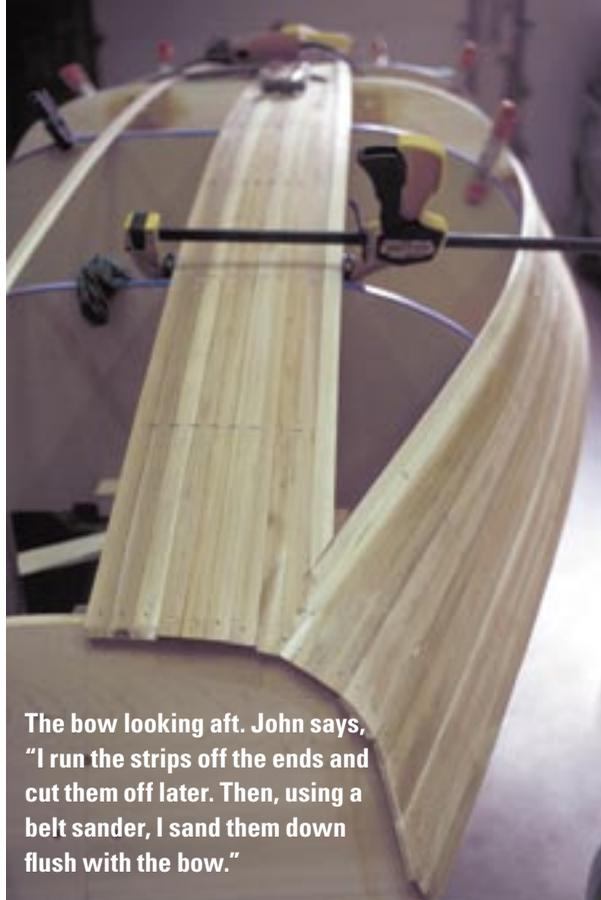
The bow looking aft. John says, "I run the strips off the ends and cut them off later. Then, using a belt sander, I sand them down flush with the bow."
