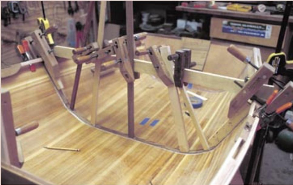
Installing the rib, at left, using a steamed piece of teak bedded down with epoxy glue then covered with a strip of fiberglass cloth. This will help keep the hull from twisting when the dinghy is rowed.
